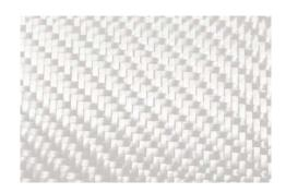
Fiberglass fabric is used in a wide range of industrial applications and is the most widely available and least expensive composite fabric. It is relatively lightweight, has moderate tensile and compressive strength and is easy to handle and machine. High strength, dimensional stability, design flexibility and excellent electrical properties are some of the characteristics that insure optimum performance.
